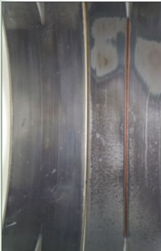
Engine main bearing halves show very little wear and are still suitable for continued use.
